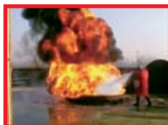
Fire test on the class 233B with 6 kg powder fire extinguisher
