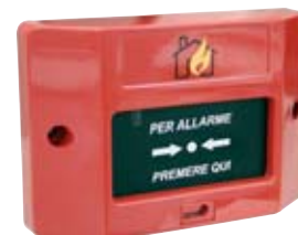
47006 Push button break glass alarm. 2 contacts n.o. and n.c. 10 A
